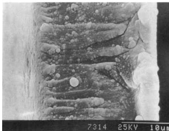
Figure 5 SEM images of cross section of the pyrolyzed polyimide films at different pyrolytic temperatures: (a) polyimide films; (b) pyrolyzed at 950°C.
